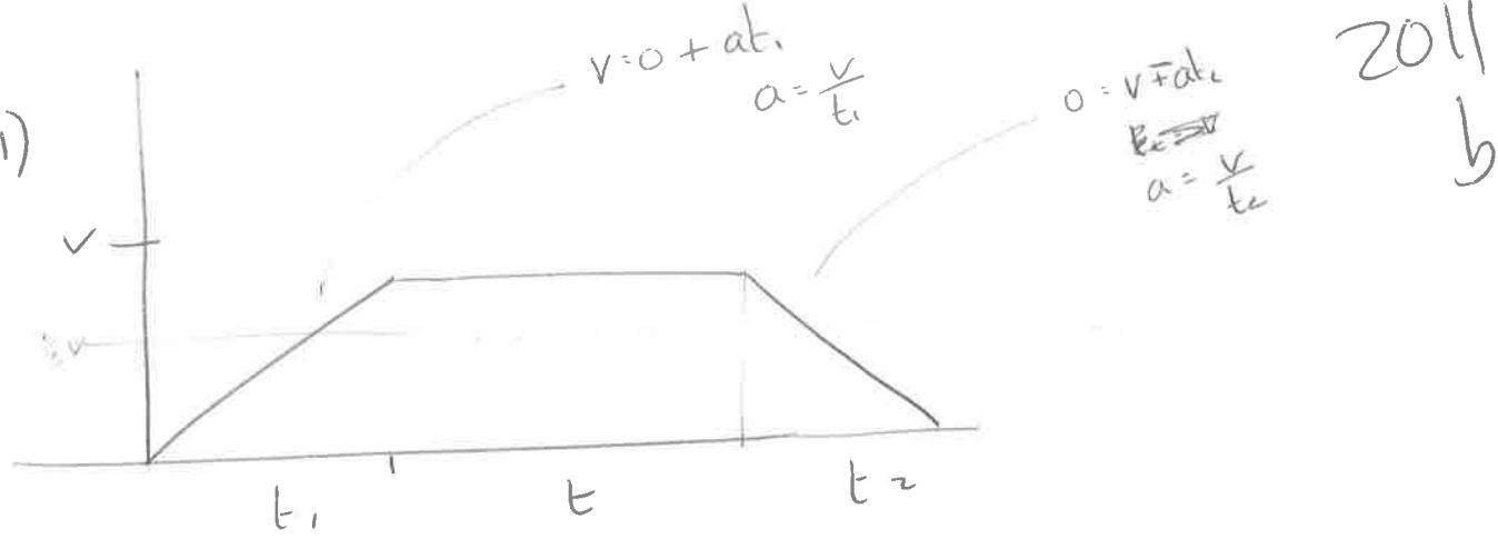
II) Av-speed =  $\frac{3v}{4} = \frac{d}{t_1+t+t+t_2} = \frac{\frac{1}{2}t_1v + tv + \frac{1}{2}t_2v}{t_1+t+t+t_2}$
